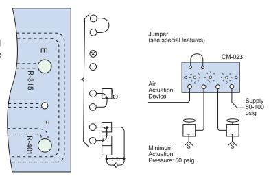
Maintained Output occurs as long as both pushbuttons are held. Release of either button terminates the output. (Connect E to F)
